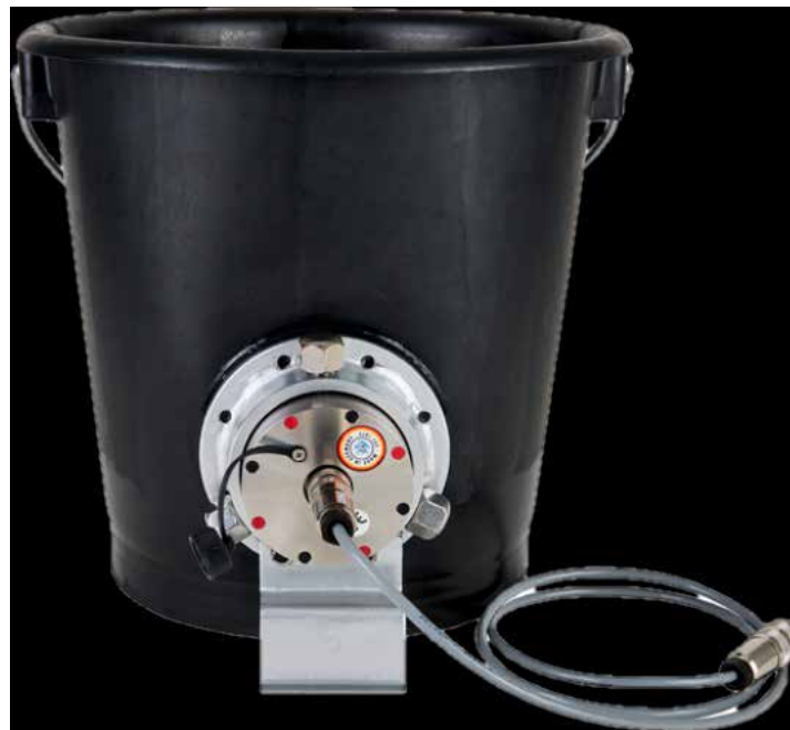
The company Franz Ludwig Gesellschaft für Mess- und Regeltechnik mbH offers in-process measurement technology for bulk goods of any kind: here, for example, the FL-Bucket Moisture Check
